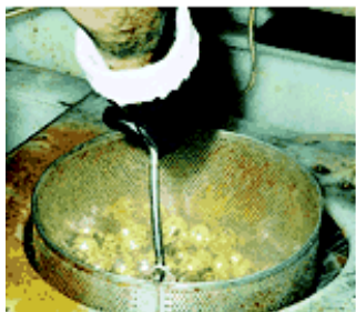
Star developed this special rinse station to ensure that each part is rinsed.
