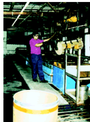
This zinc plating line is a manual hoist system.
