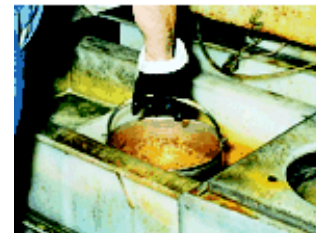
After rinsing, the parts are dipped in the brass dye solution.
