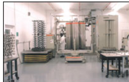
Physical vapor deposition (PVD) is one of several finishing processes offered by ECF's Remico plant. PVD applies a thin metallic finish to the parts, imparting a variety of colors from gold to silver.
